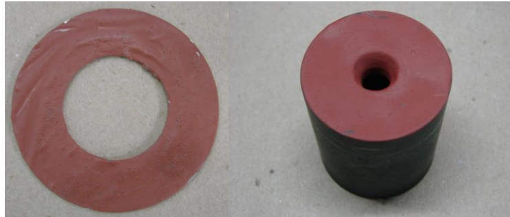
Figure 11. Left: Painted ring to prevent nozzle deterioration. Right: Painted nozzle prior to firings.
