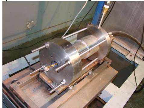
Figure 9. Upper side view of the lab-scale hybrid rocket motor on the test bench.
