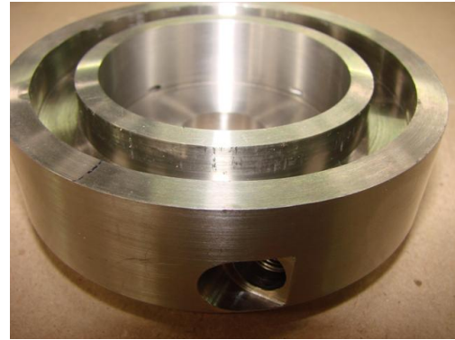
Figure 6. Lateral view of the large swirl without the connectors and hoses.
