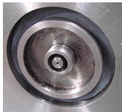
Figure 4. Injector mounted in the test bench.
