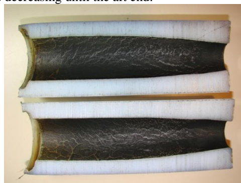
Figure 11. Grain cross section after axial injector test.
