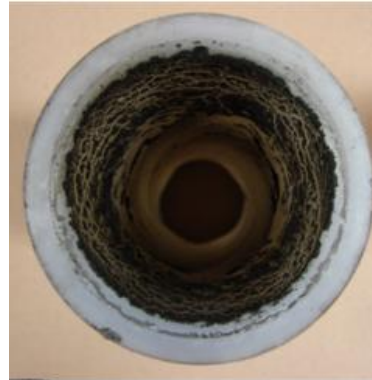
Figure 13. Grain superior view obtained from the small swirl injector test.
