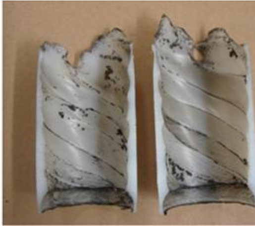
Figure 16. Grain cross sectional view after large swirl firings.
