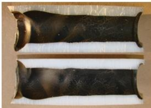
Figure 14. Grain cross section after axial combined with small swirling injectors test.
