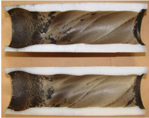
Figure 12. Helicoidally disposed curves on the grain surface subsequent to small swirling injector test.
