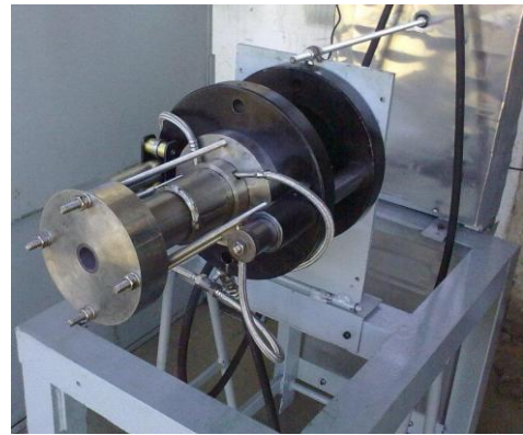
Figure 2. Picture of the hybrid rocket motor configuration.
