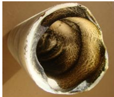
Figure 15. Grain superior view. Helicoidally disposed imprints along the axis obtained after axial and small swirling injectors test.
